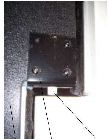
Door Panel Bottom Hinge Pivot & Guard
